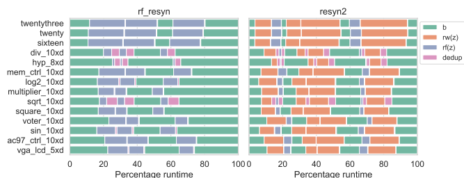
Fig. 8: Runtime breakdown of GPU rf_resyn and resyn2 .
